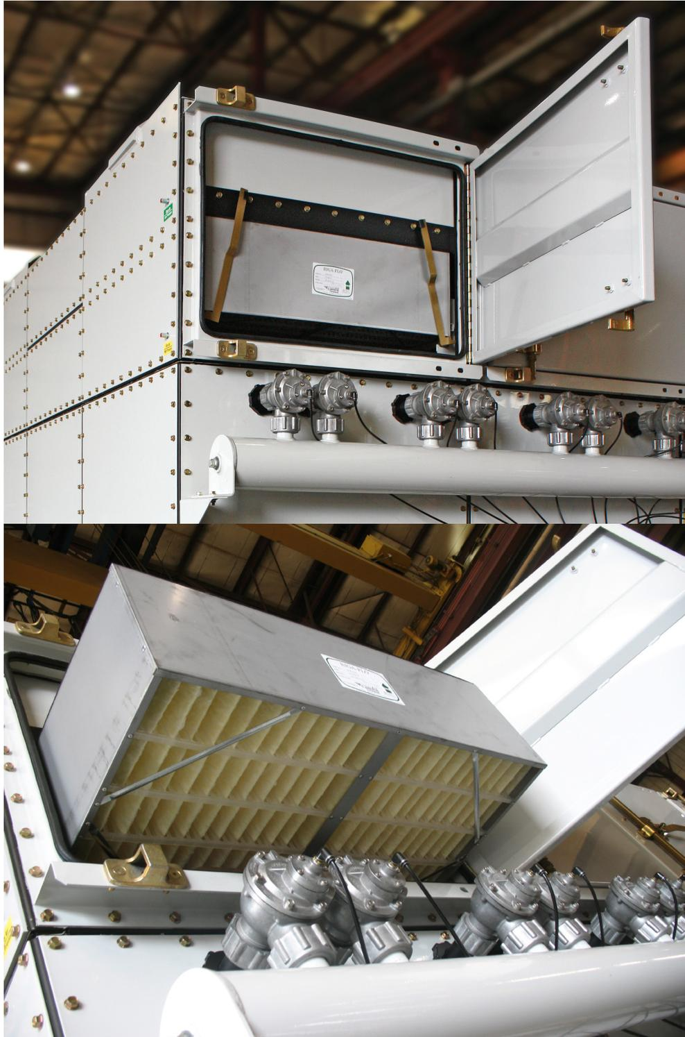
**The iSMF is provided by Camfil APC factory installed.** There are very few items that need to be verified prior to start up commissioning. These items should be inspected prior to start up, after filter replacement and annually as part of your routine inspection and maintenance program for equipment handling combustible dusts.
