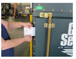
Figure 400.10.7 - Add additional shims for any other areas that require gasket compression. Re-test all areas after adding shims.
