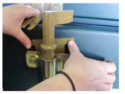
Figure 400.10.5 - Loosen bolts and insert one shim
