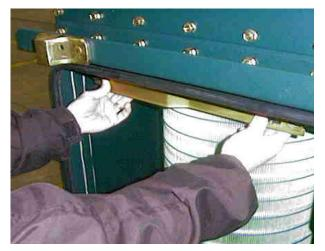
Figure 230.1.1 - Clamp bars closed
