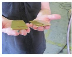
Figure 400.10.4 - Use either 1.5 mm. Or 3 mm shim (the unit comes with 2 of each)
