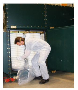
Figure 230.2.2 - Put the plastic bag under the used cartridge
