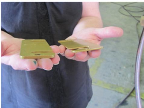
Figure 400.10.4 - Use either 1.5 mm. Or 3 mm shim (the unit comes with 2 of each)
