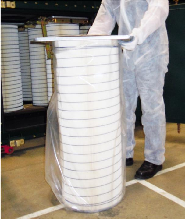
Figure 230.2.5 - Pull out the cartridge
