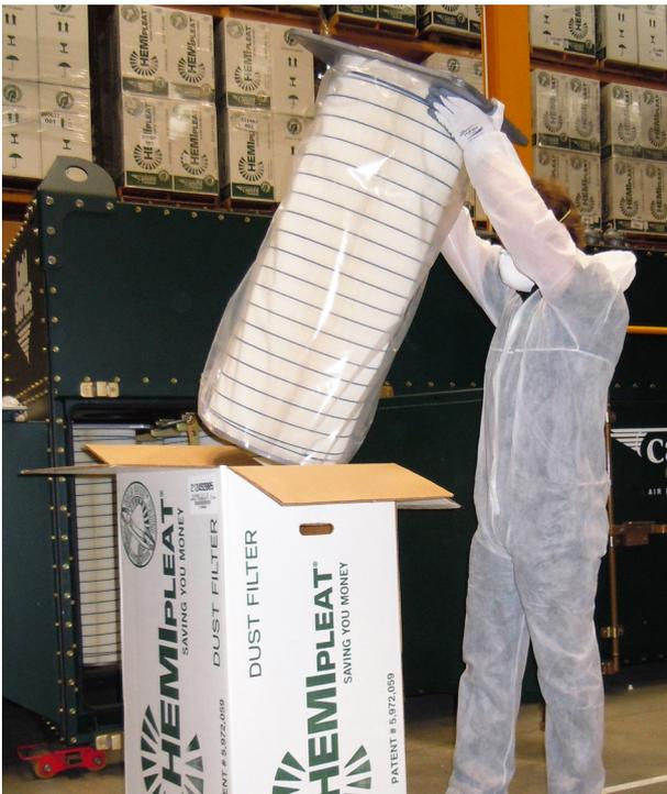
Figure 230.2.6 - Place the used cartridge in the box that came with the replacement cartridge
