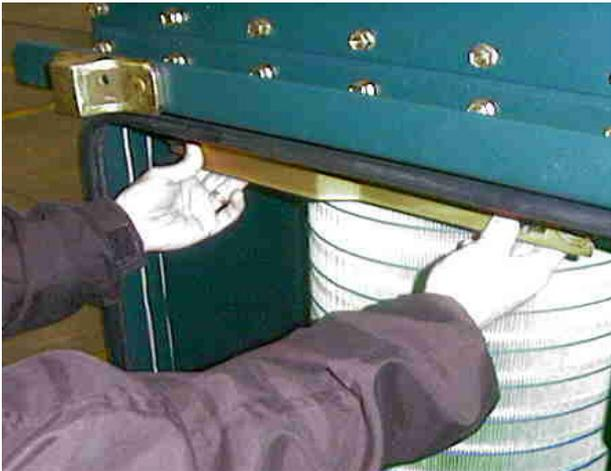
Figure 230.1.1 - Clamp bars closed
