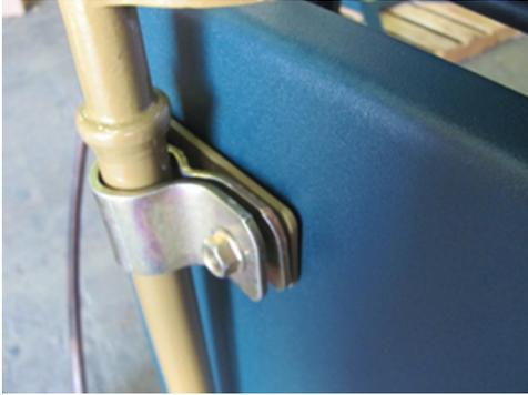
Figure 400.10.6 - Verify shim is in place and retighten bolts
