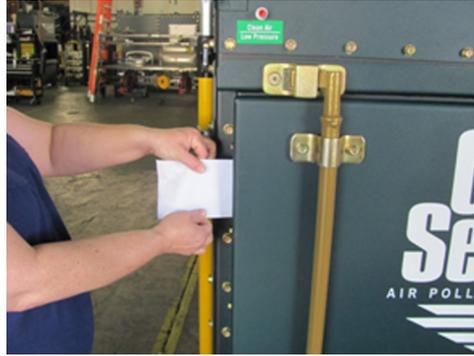
Figure 400.10.7 - Add additional shims for any other areas that require gasket compression. Re-test all areas after adding shims.
