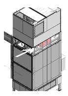
► Push the new filter elements into the separator housing.
