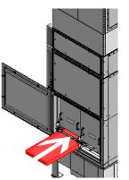
Insert the cleaned or new filter element in the separator housing.
