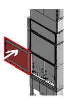
► Open the maintenance door with an 8 mm Allen key.
