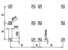
Mounting according to the drilling template (separate dimension sheet)
