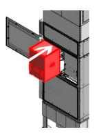
► Slide all filter elements up to the stop in the separator housing.
