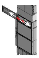
► Fold the clamping lever sideways, right and left from the inside out.
