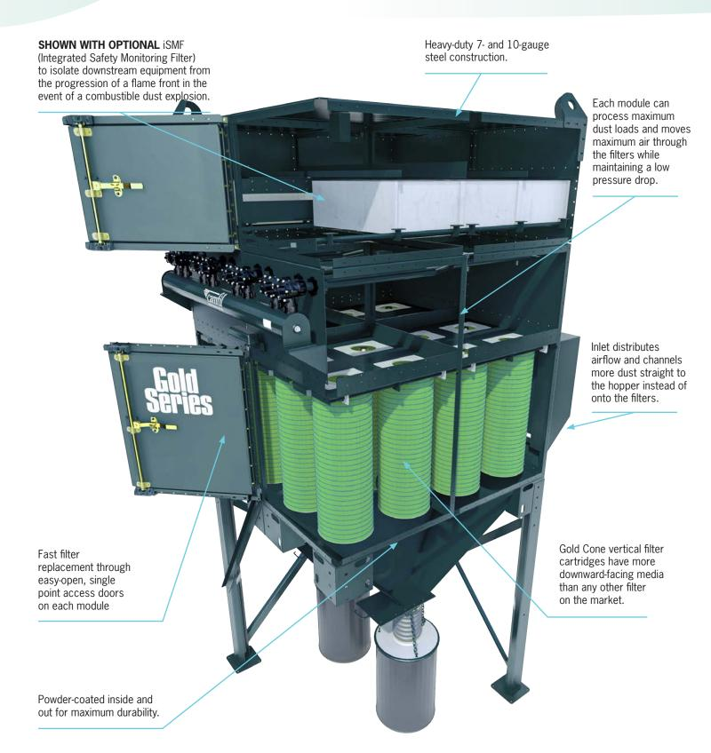
Combustible dust explosions pose a significant risk at many manufacturing, processing and metalworking plants. One of the leading causes of such incidents is an unprotected dust collection system. Gold Series dust collectors help reduce these risks by being customized to your specific situation.
