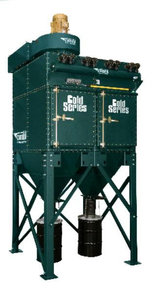
Gold Series collectors feature a modular design for optimum field flexibility. Each module accommodates airflows up to 4,000 cfm using four cartridges mounted in a symmetrical frame. Additional modules may be added to meet total airflow requirements of 100,000 cfm and beyond.
