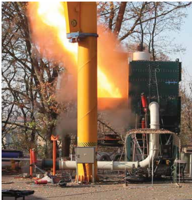
A staged explosion is used to test a dust collector's ability to withstand a combustible dust event.
