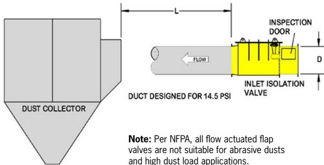
**Note:** Per NFPA, all flow actuated flap valves are not suitable for abrasive dusts and high dust load applications.
