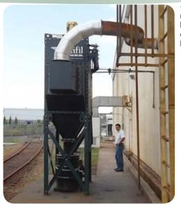
▲ A view of the replacement: a GS8 Farr Gold Series dust collector with HemiPleat cartridges.
