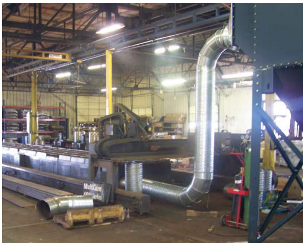
Farr Gold Series® model GS16 removing dust and fumes from a plasma table.
