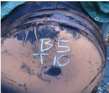
Uniform blade deformation from explosion tests. Note, this is the 5th blade consumed in 10 tests. It is highly probable that your valve will survive an explosion activation.
