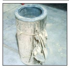
Competitor's cartridge "blown out" under the pressure.
