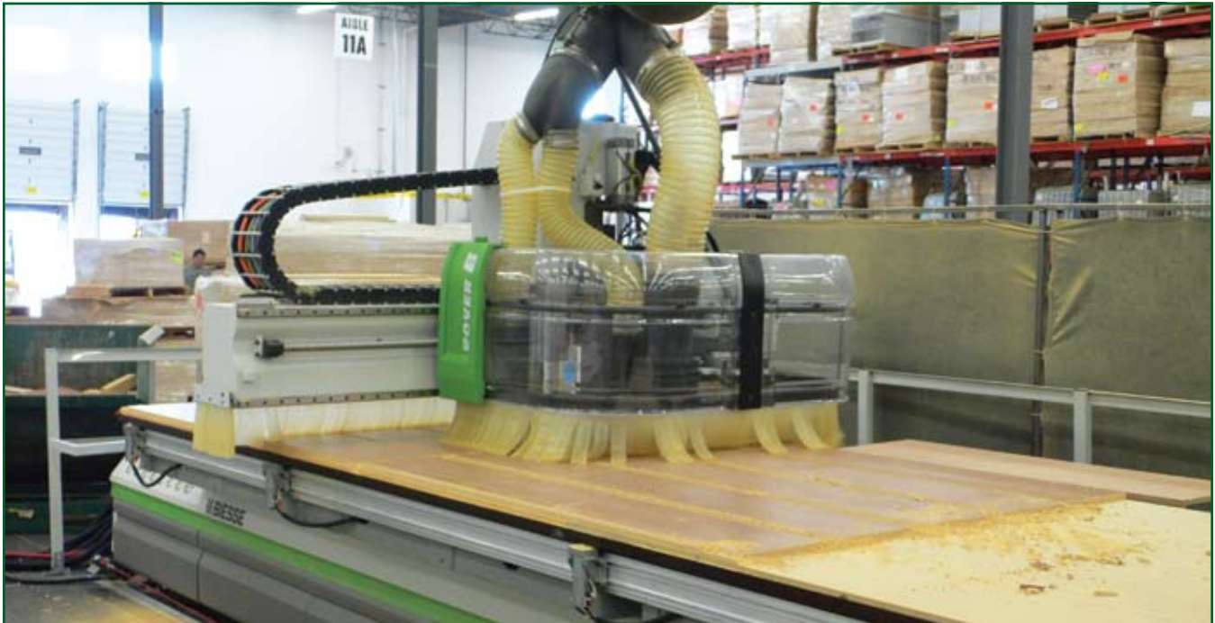
A router exhaust hood is connected to the exhaust system.
