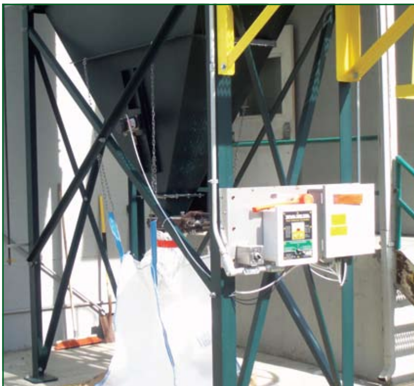
This pyramid hopper features a special mounting bracket for a vibrator to aid in material flow.
