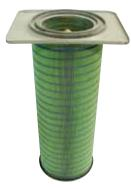
Camfil Farr APC Gold Series® cartridges have an expanded capacity due to the patented inner Gold Cone™. This inner cone increases media area and provides uniform dispersion of back-pulsed air. It also opens up more usable space for air flow in the filter.
