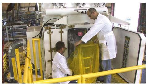
The Camtain solution comprising BIBO for safe filter changes and continuous bin liner for safe waste product collection and disposal.
