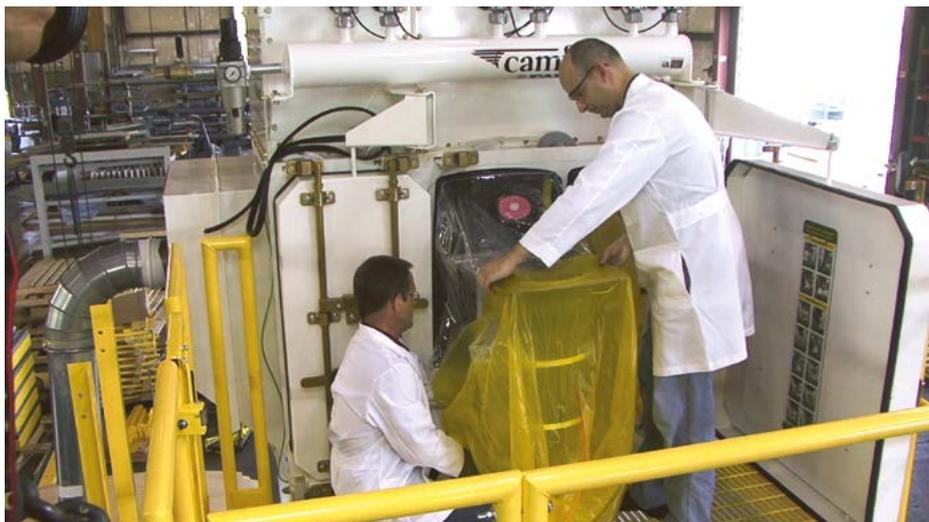
The Camtain solution comprising BIBO for safe filter changes and continuous bin liner for safe waste product collection and disposal.
