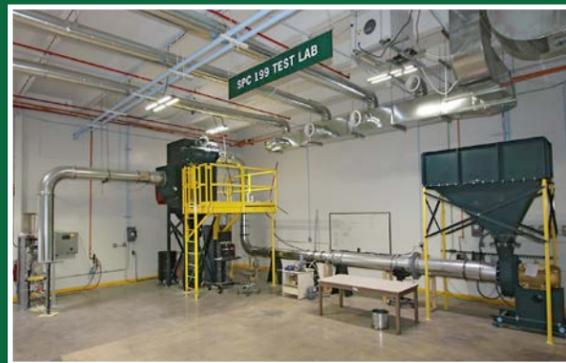
ASHRAE Standard 199 Dust Test Apparatus
