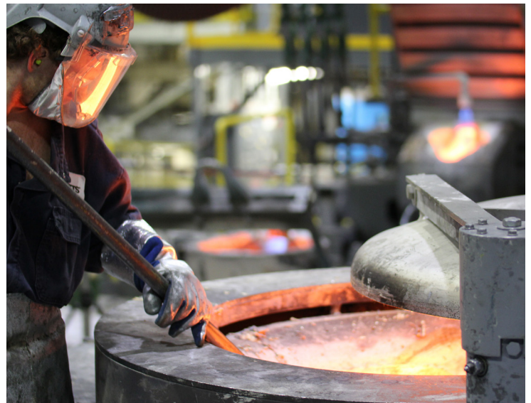
▲ Fumes from melting metal are collected at the source.
