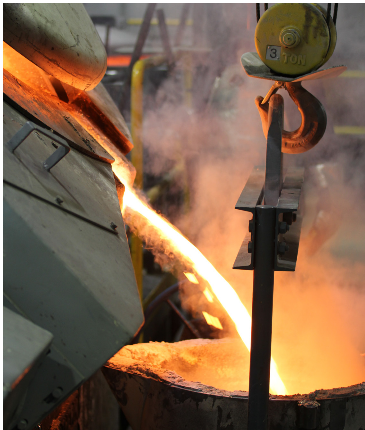
▲ Fumes from liquid metal being poured for transfer in the new foundry.
