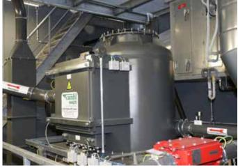
High-pressure vacuum filter for extraction of dust and chips
