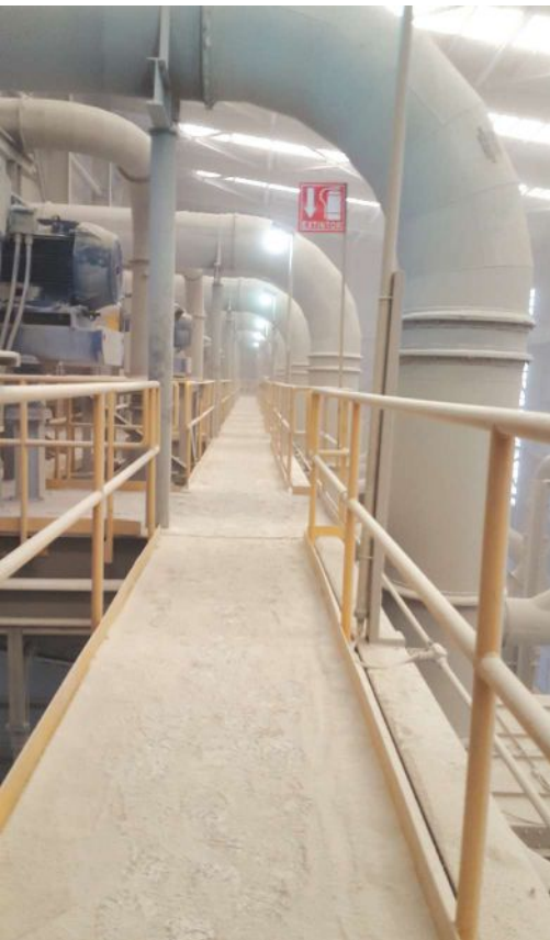
Fugitive dust emissions not only represent a safety hazard, but a loss of valuable product.
