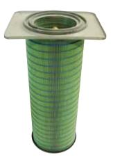
Camfil Farr APC Gold Series<sup>®</sup> cartridges have an expanded capacity due to the patented inner Gold Cone<sup>™</sup>. This inner cone increases media area and provides uniform dispersion of back-pulsed air. It also opens up more usable space for air flow in the filter. The lead dust is collected in a standard 210 litre drum for easy disposal and the hopper is fitted with a shut off valve to ensure there is no leak-age of dust when the drum is being changed.
