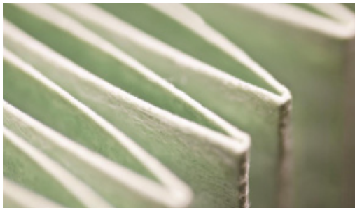
Wide-pleat style cartridge filter media
