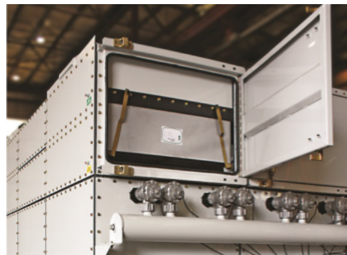
HEPA-grade integrated secondary monitoring filter (iSMF)
