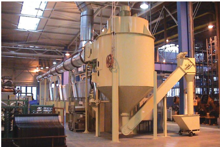
“Venturi scrubber”: This venturi-type wet scrubber is used for combustible dust control in an automotive-parts manufacturing plant.
