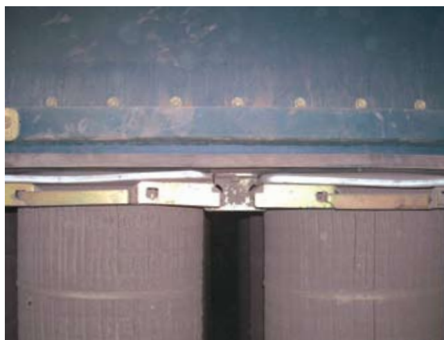
Warped mounting plates encourage gasket leaks.
