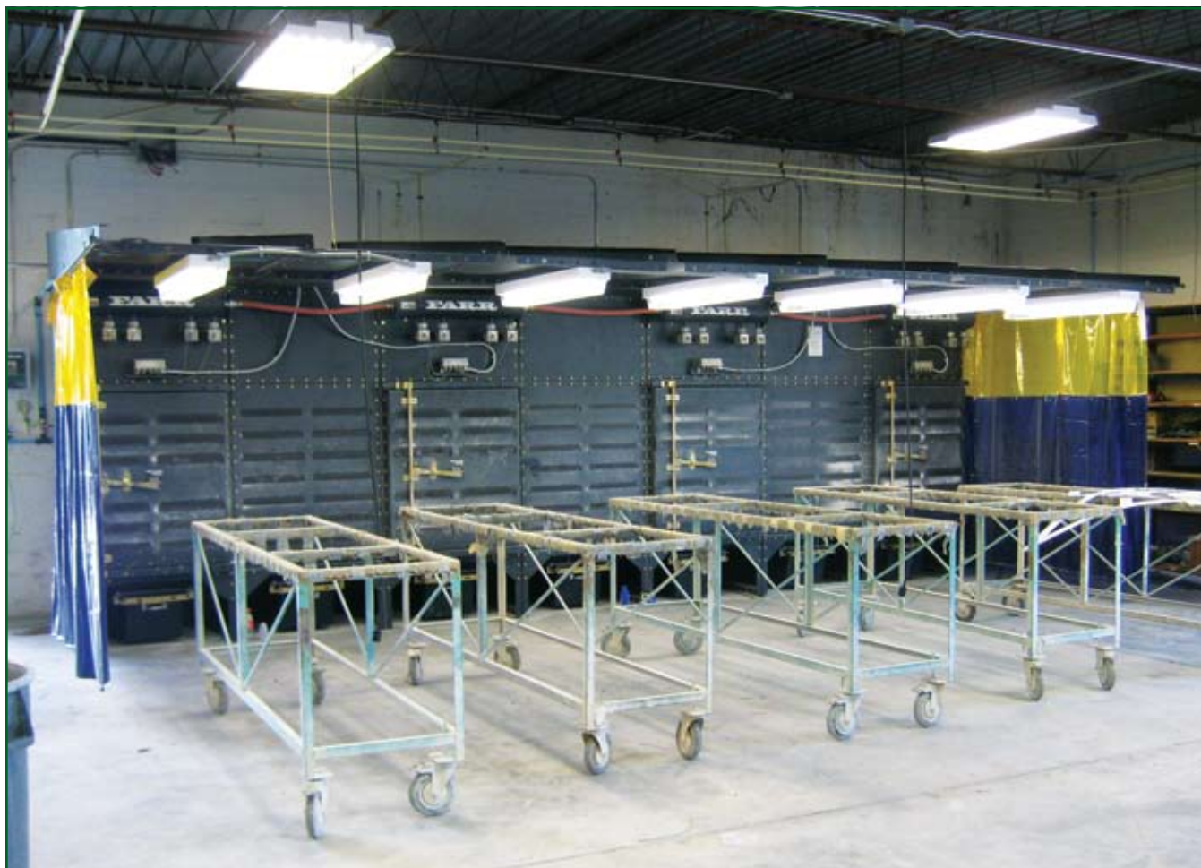
21,600 CFM Gold Series Booth encapsulates blast dust in countertop manufacturing area.
