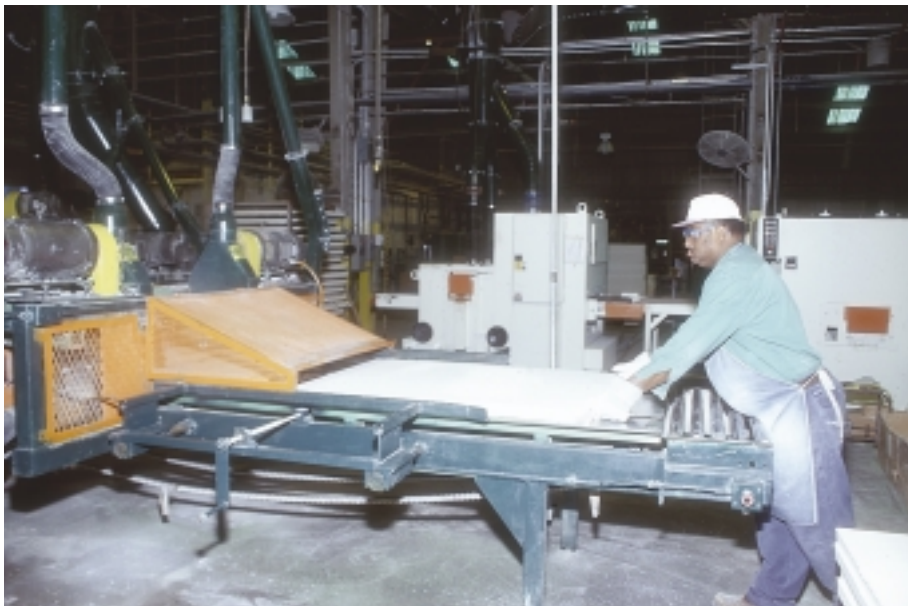
Operator Robert Gilchrist loads boards onto the inlet rollers for the cross-cut saw.
