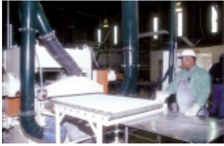
Operator Robert Gilchrist watches as boards are discharged from the planer-sander.
