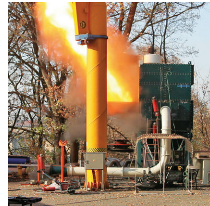
An engineered test is performed at an official testing facility to confirm that this dust collector can withstand an explosive event. Scan QR code to view brief explosion test video.
