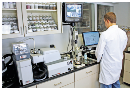
Bench testing identifies physical properties of the dust, aiding filter selection.
