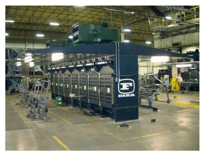
tion of multiple Farr Gold Series Booths (GSB's) with HemiPleat™ filters. The GSB's would enclose and isolate each of the 10 workstations and occupy a minimum of valuable floor space.
