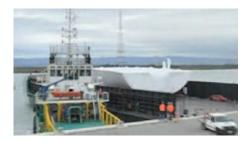
Each ship is manufactured in single "blocks" before completion.
