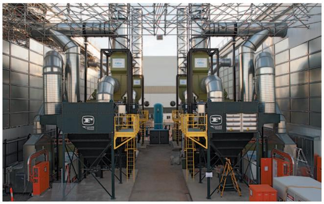
Four Farr Gold Series dust collectors with explosion vents are located between the two temporary buildings with no interference with surrounding equipment.
