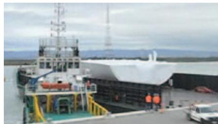
Each ship is manufactured in single “blocks” before completion.
