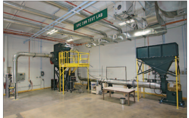
This full-scale test rig, built in accordance with Standard 199 specifications, includes a cartridge dust collector with four high-efficiency filters.
