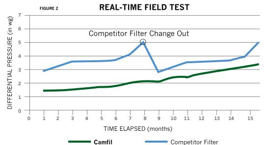
Field testing provides real life data that Camfil HemiPleat cartridges have a lower pressure drop and last longer. Figure 2 shows a 16-month test in two competitor's collectors. One unit had Camfil HemiPleat cartridges and the other had a leading competitor's brand installed. In these identical real-life processes, the competitor's cartridges started at a higher pressure drop and required a filter change at eight months, while the Camfil cartridges were still performing at a 2" pressure drop.
