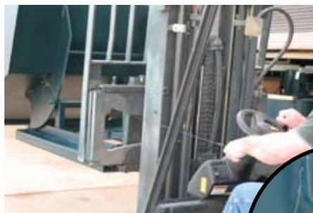
When the hopper is full, the user detaches it from the bottom of the collector, lifts the hopper onto a fork truck, and simply pulls a lever to swing the lid open and dump the contents into a larger disposal container.
