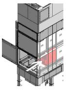
► Insert the cleaned or new filter element in the separator housing.
