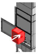
► Slide all filter elements up to the stop in the separator housing.
