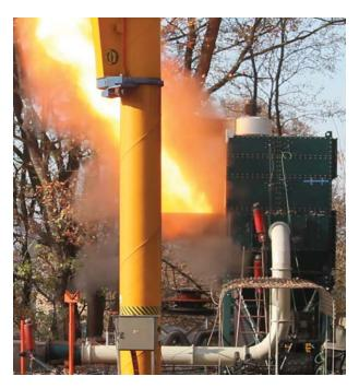
An engineered test is performed at an official testing facility to confirm that this dust collector can withstand an explosive event. Scan QR code to view brief explosion test video.
