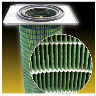
Open-pleated media allows the collected dust to release from the filter, keeping the resistance lower through the filter and extending filter life. Exploded view shows internal pleat separation technique.
