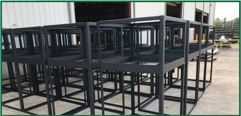
Modular construction of Gold Series dust collectors
