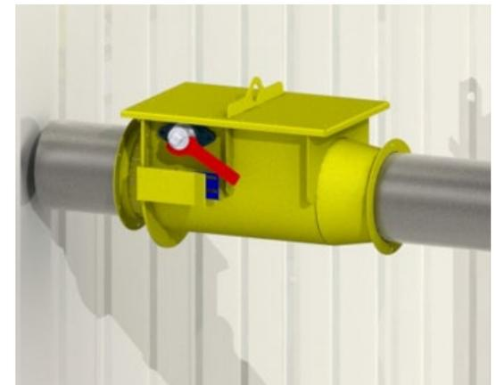
A self-adjusting latching mechanism engages when the valve closes and holds the valve shut during the deflagration. This mechanism will not engage during normal shutdown of the system fan.
